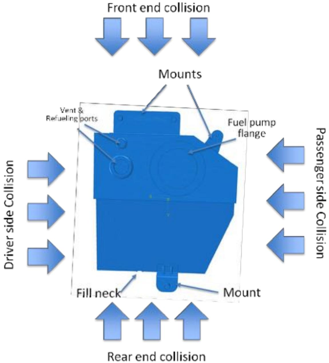
Figure 2: Fuel tank geometry with the direction of acceleration due to different collisions.
