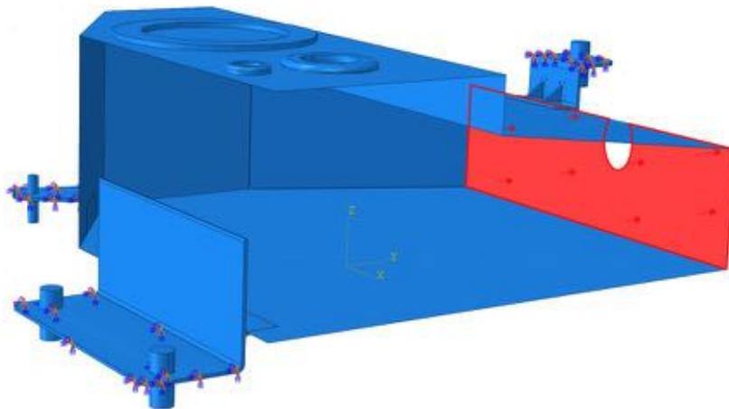
Figure 10: Pressure due to impact from fuel.
