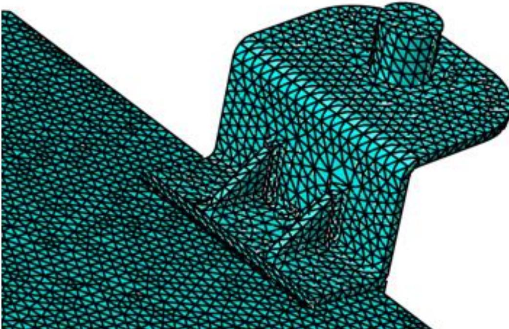
**Figure 6: Rear mount meshed attached to the meshed tank.**
