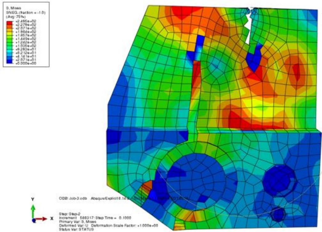
Figure A 1: Tank without brackets, damage from 50 mm displacement
