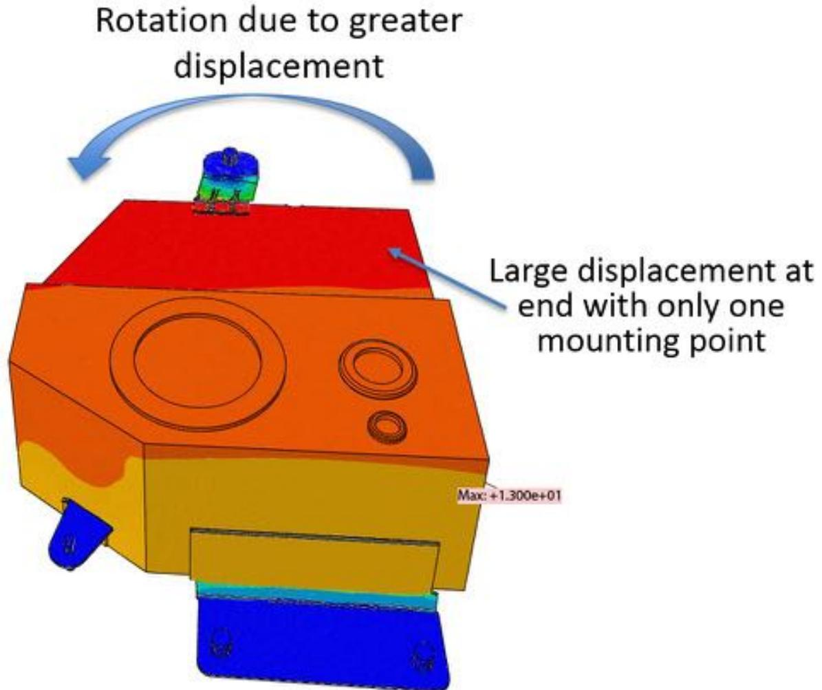
**Figure 18: Visualizing the displacement of the tank during passenger-side collision**
