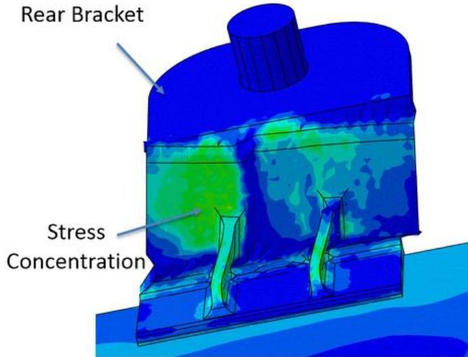
Figure 16: Rear bracket during passenger-side collision
