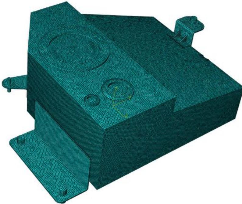
Originally, the tank was meshed using rectangular blocks, or a quad type, since the mesh best suited the geometry. This type of mesh proved to be problematic when tying the mounts to the tank because the mesh geometry didn't agree. To resolve this issue, a tri-type mesh was used with a global seed size of 4 as seen in Figure 3. The tank took the most elements to create its mesh – almost 95,000 elements.
