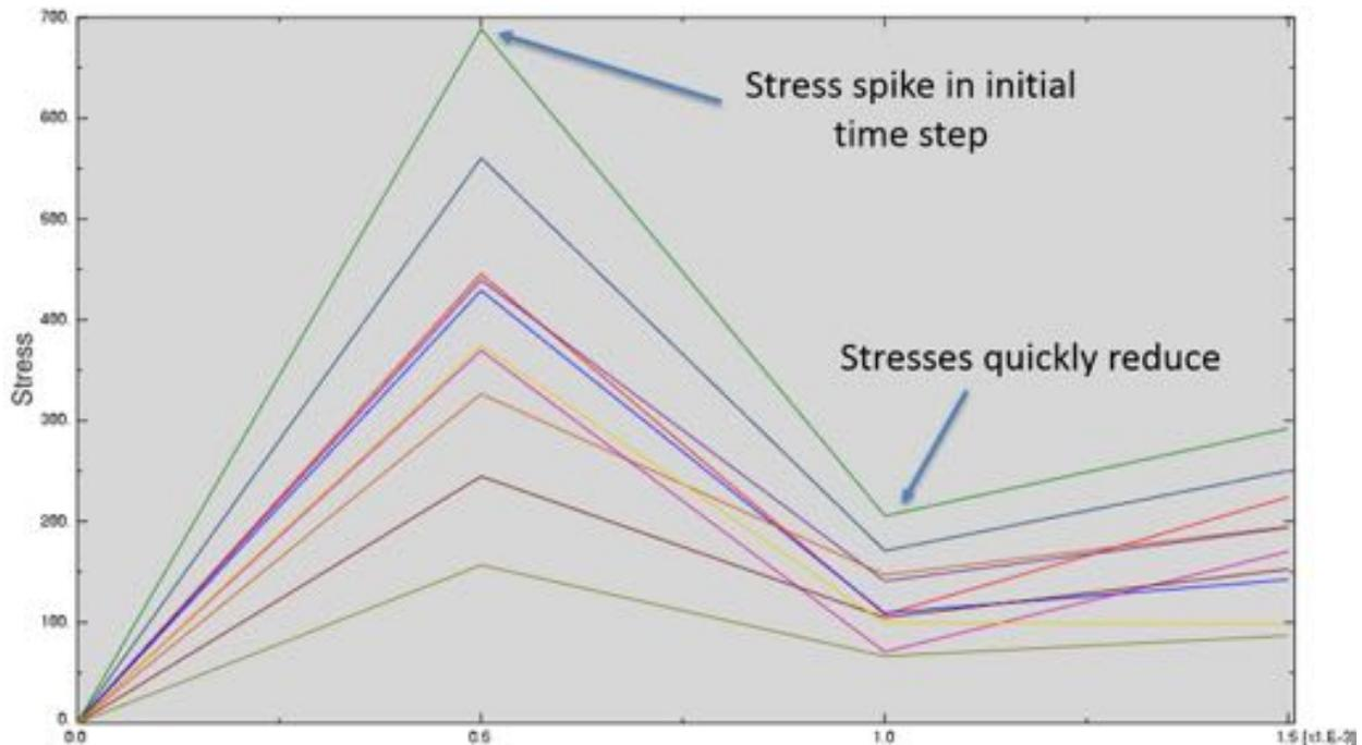
Figure 12: Spikes in stresses due to constraints.
