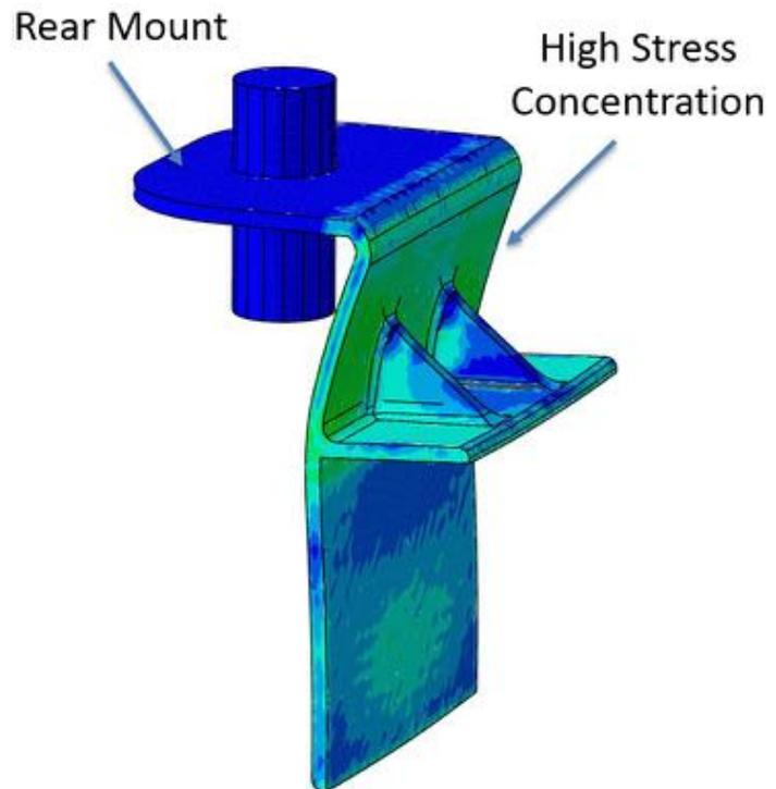
Figure 17: Rear bracket during a rear-end collision
