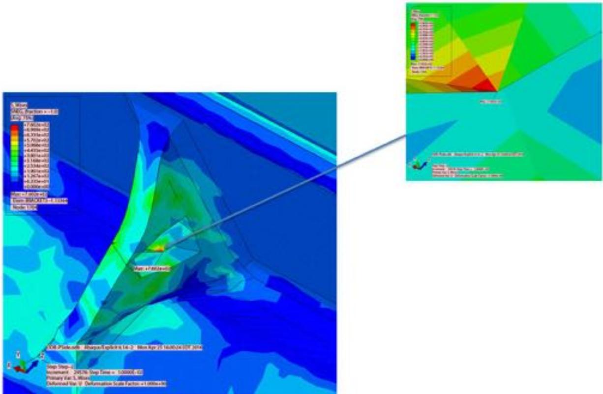
Figure B 1: High stress element within supports
