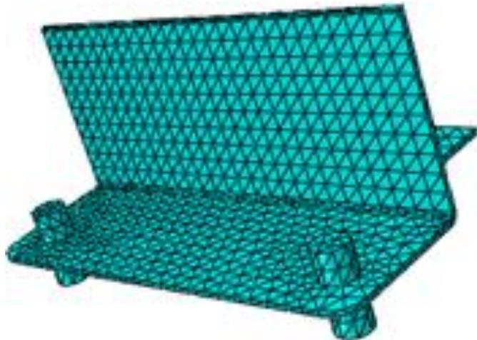
Figure 4: Front mount meshed with tetrahedral elements.
