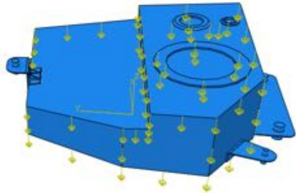
Figure 8: Acceleration due to gravity on the mass of the tank.
