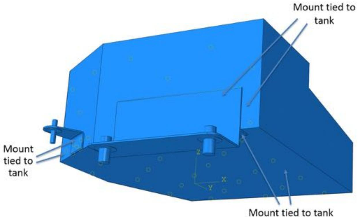
Figure 11: Tying the brackets to the tank.
