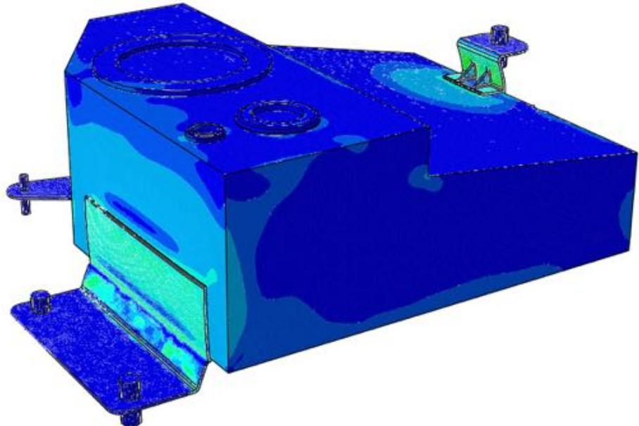
Figure 15: Rear-end collision simulation.
