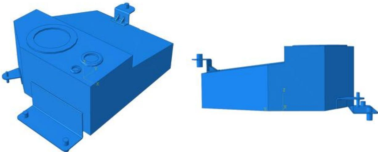
**Figure 1: Geometry of the hybrid fuel tank designed.**
