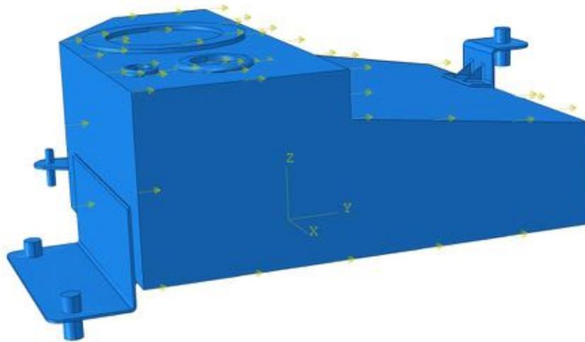
Figure 9: Acceleration due to rear-end collision.
