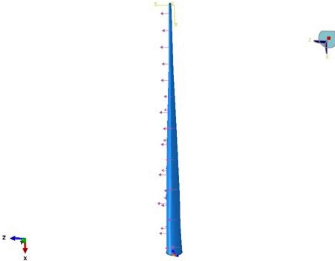
**Figure 7:** Distributed Wind Loading Condition
