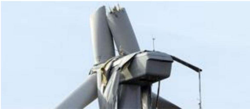
**Figure 1:** Blade Failure in a Wind Turbine Blade [3]
