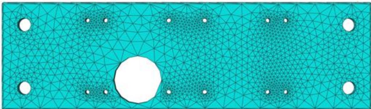
Figure 6: Simplified Plate Mesh
