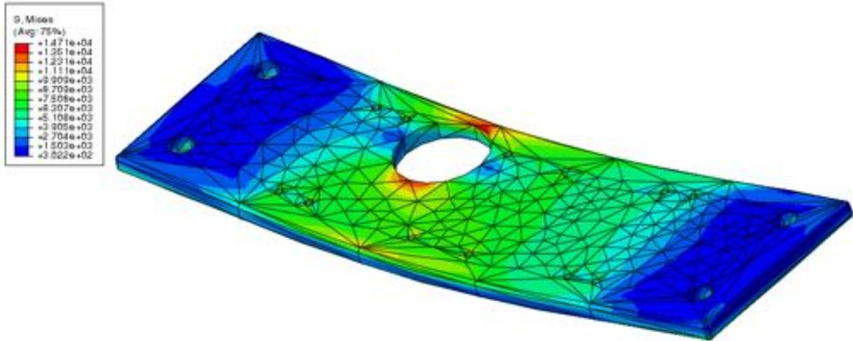
Figure 22: Von Mises Stress Plot of Main Plate
