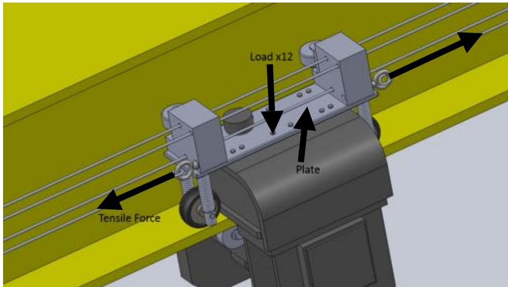
Figure 1: Trolley Assembly with Applied Loads
