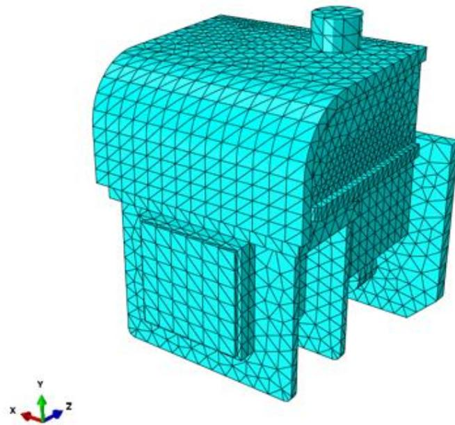
Figure 13: Slider Mesh Opposite View
