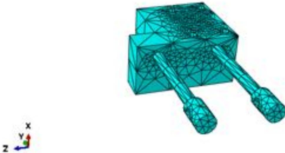
Figure 9: Shock Mesh Underside
