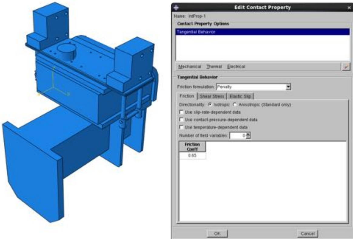
Figure 19: Friction Application
