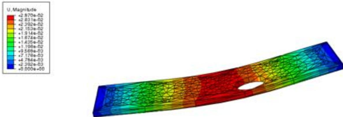
Figure 23: Deformation Plot of Main Plate
