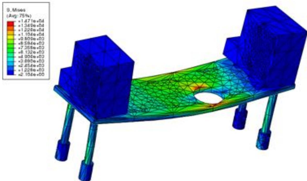
Figure 21: Von Mises Stress of Assembly
