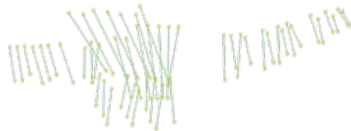
Figure 8: Highlighted ligament slave tie nodes. The end nodes of each ligament were tied to their corresponding master node on the vertebra body
