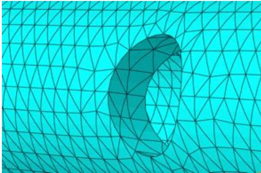
**Figure 4: 10-016 Meshed Strut**
