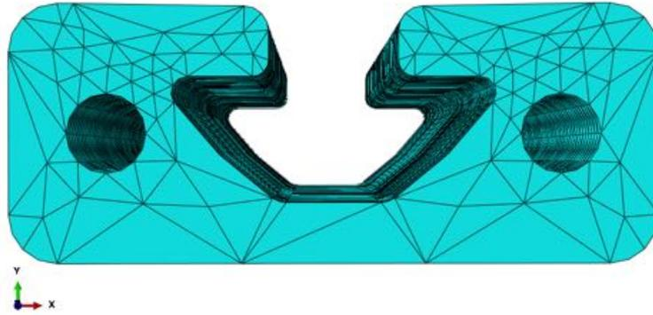
**Figure 6: 10-081 Meshed Strut**
