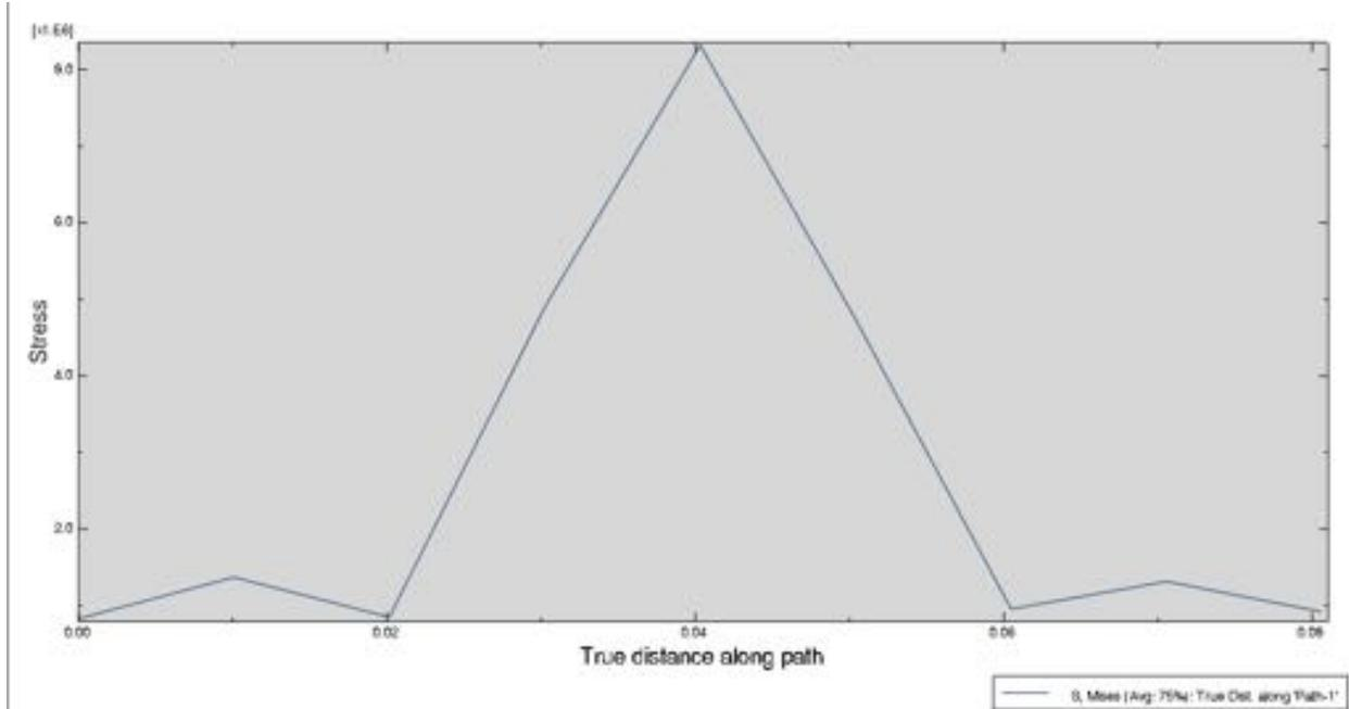
Figure 21: Stress around the circumference of the Mount Tube base
