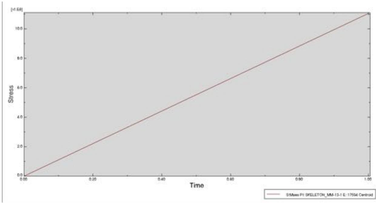
Another method used to visualize how the stress of an element changed over the loading time was to plot the values obtained at the integration points of the element, also known as the Gauss points. These are the points where the stresses obtained from the nodal values of the element are transferred to the Gauss points using the elements shape functions. Figure 18 shows how the four Gauss points of a tetrahedral element change over the loading time.
