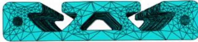
**Figure 8: Meshed Mount Tube Ring**
