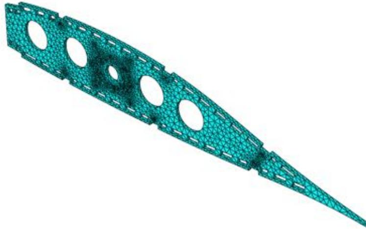
**Figure 10: Final Meshed Assembly**
