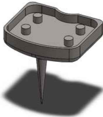
Figure 7: Imported CAD geometry of the tibial implant.
