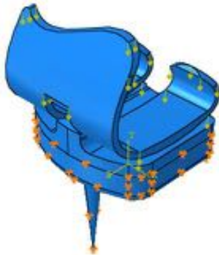
Figure 13: Cyclic load is applied to the femoral implant.
