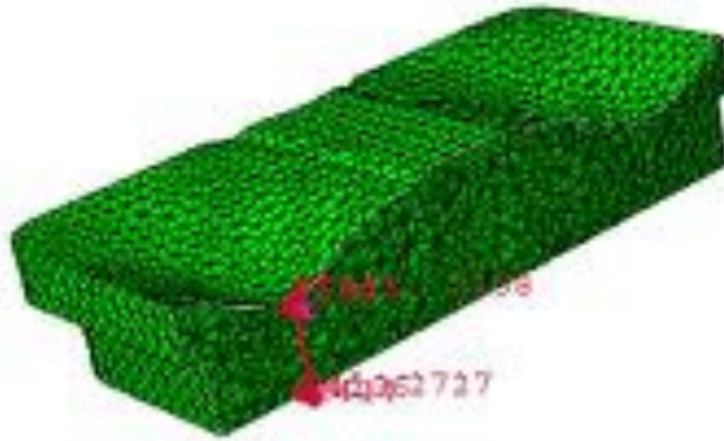
Figure 21: Cutaway view of meniscus highlighting the path that the stress XY data was measured at.
