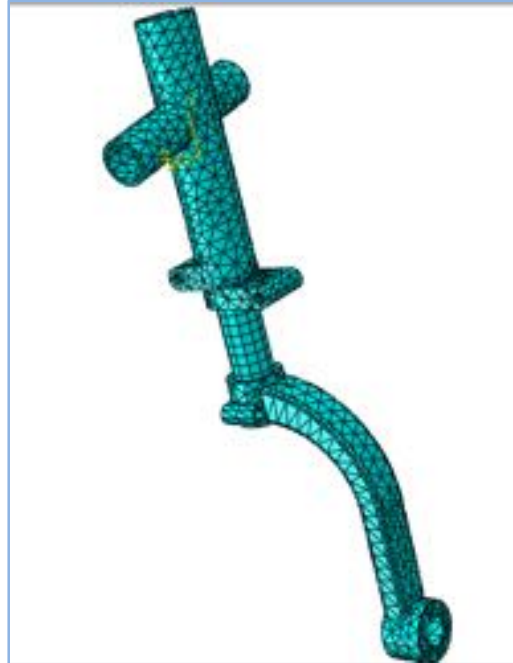
Figure 9: The complete assembly of all landing gear parts with the mesh displayed.
