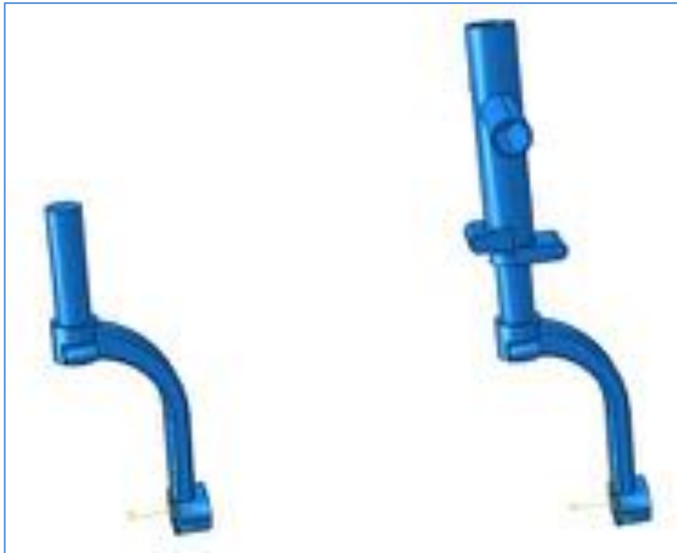
Figure 8: The landing gear fork and cylinder assembly (left) and the complete assembly of the landing gear (right).
